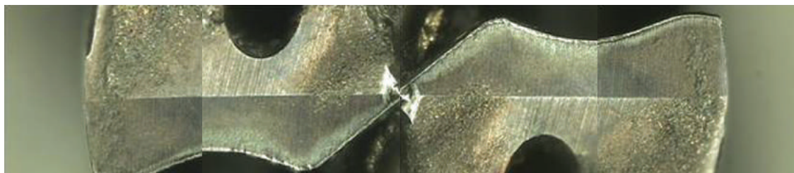
COMPETITOR A (After Drilling 546 Holes)
