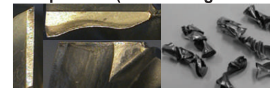
Competitor A (Total Drilling 80 Holes)
