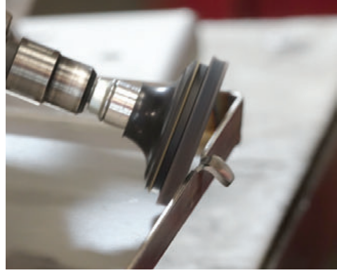
Edge chamfering a fabricated stainless steel component.
