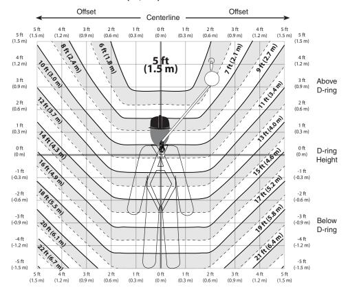
**EXAMPLE:** With the SRL-LE anchored 4 feet above the users D-ring and the user works 2 feet away (offset) from directly overhead (centerline), the required clearance is 6 feet (1.8 m) from the working level to the nearest obstruction below.
