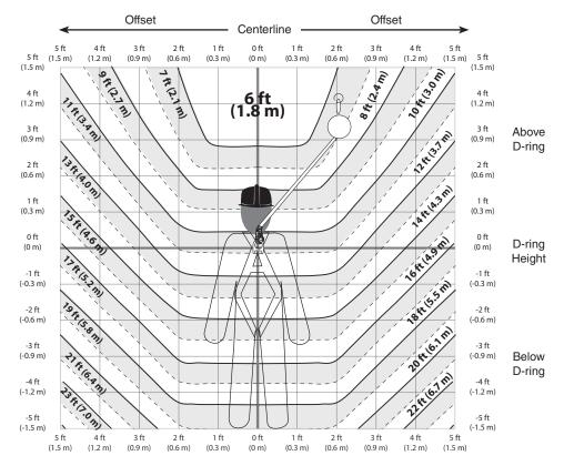
**EXAMPLE:** With the R410065LE anchored 4 feet above the users D-ring and the user works 2 feet away (offset) from directly overhead (centerline), the required clearance is 7 feet (2.1 m) from the working level to the nearest obstruction below.
