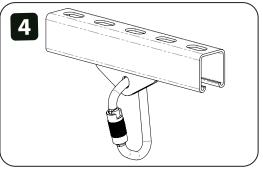
4. Connect to the anchorage connector using a carabiner going through both holes of the anchorage connector. PFAS must limit fall arrest forces to 1800-lbs (8 kN) or less.
