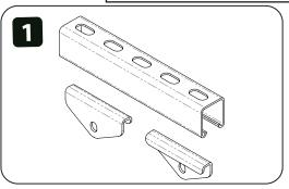
1. Choose location in Strut Channel. A qualified person must determine if a specific installation location will meet all ANCHORAGE REQUIREMENTS. Insert the two pieces of the anchorage connector into the strut channel.
