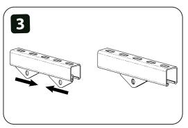
3. Bring the two pieces of the anchorage connector together.
