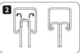
2. Hook both sides of the anchorage connector onto the strut channel. Both pieces of the anchorage connector must be used. DO NOT USE the anchorage connector without both pieces.
