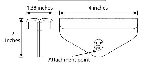
Minimum Breaking Strength (MBS): 5,000-lbs (22kN)
