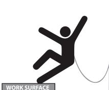
\*The structure the receptacle is attached to must be able to support 5,000-lbf (22kN) and installed under the supervision of a qualified person.
