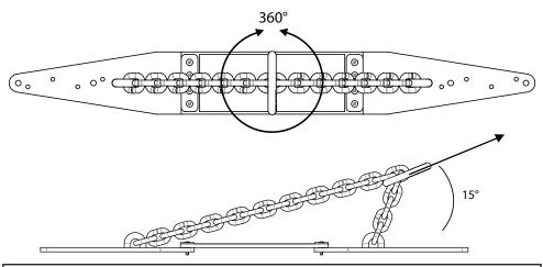
When installed with six M6 x 80mm grade 2 lagbolts or six ¼ inch x 3 inches grade 2 lag bolts the anchorage connector is rated for loading at 360° (horizontally) and up to 15° (vertically) as shown in the LOADING CONDITIONS DIAGRAM. Loading at any angle outside of this range is not permitted and may result in anchor failure. *Misuse or failure to follow warning and instructions may result in serious personal injury or death.*
