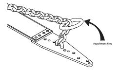
3. Connect personal fall arrest system (PFAS) to Attachment Ring. PFAS must limit fall arrest forces to 1800-lbs (8KN) or less.
