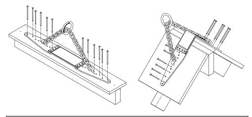
2. For installation with nails, drive in twelve 16D 3-1/2 inch spiral nails. The head of each nail should lie flush with the anchor plate. Installation for PFAS with nails creates an OSHA compliant 3,600-lbs anchorage connector within the intended direction of loading.
