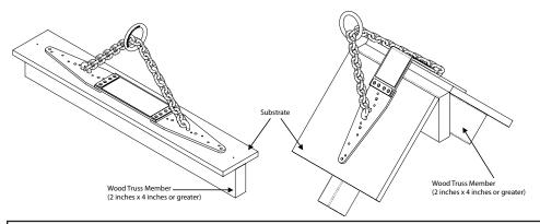
1. Choose a location either on the field or over the roof ridge at least 6 feet from the roofs edge and directly over a wood truss member\* where all holes will allow fastener penetration through the sheathing substrate to the truss below. A qualified person must determine if a specific installation location will meet all ANCHORAGE REQUIREMENTS.
