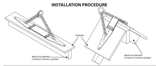
1. Choose a location either on the field or over the roof ridge at least 6 feet from the roofs edge and directly over a wood truss member\* where all holes will allow fastener penetration through the sheathing substrate to the truss below. A qualified person must determine if a specific installation location will meet all ANCHORAGE REOUIREMENTS.
