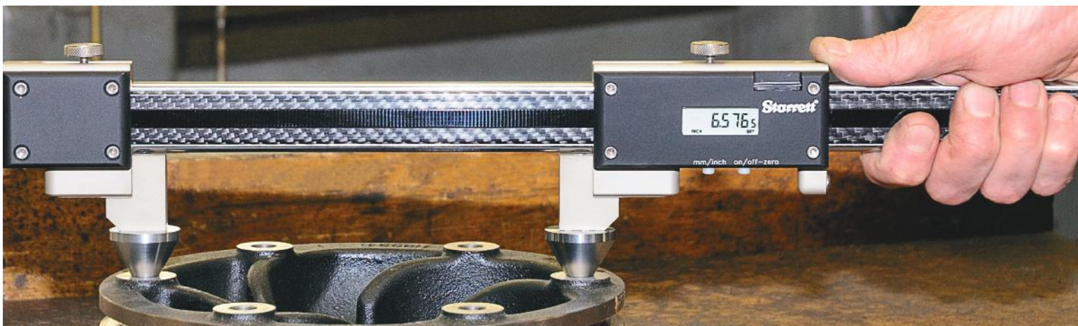
5002BZ-40/1000 with PT06137 Disc Contacts
