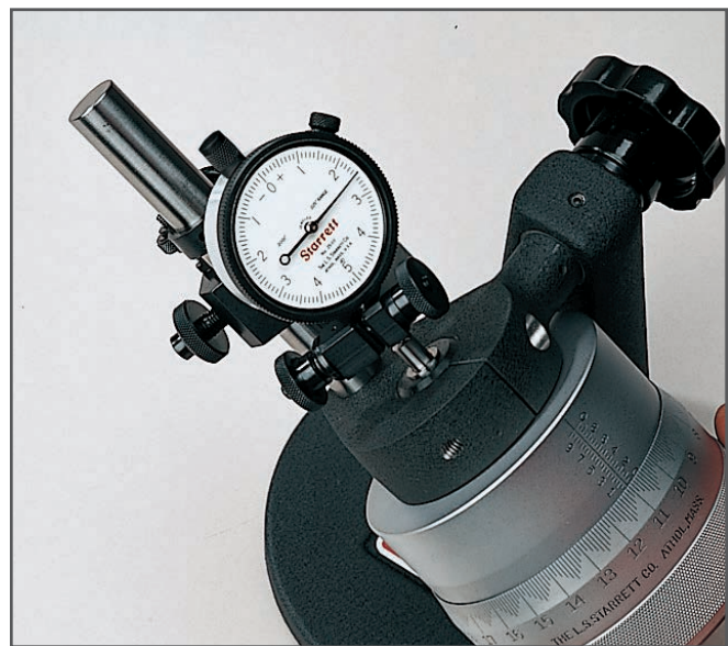
Checking AGD dial indicator
