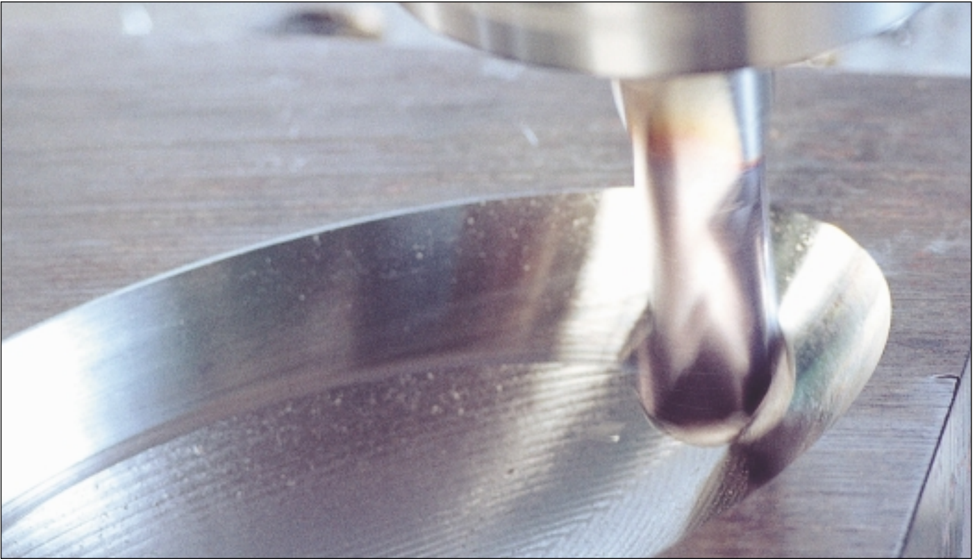
The term High Speed Machining (HSM) commonly refers to end milling at high rotational speeds and high surface feeds.
