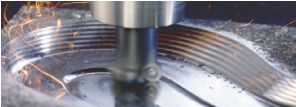
Coromant ball nose endmills, round insert cutters like the CoroMill 200 /300 and CoroMill Plura carbide endmills with large corner radii are suitable for hard steels.
