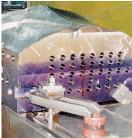
Coolant holes in a mold base.
