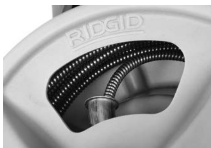
Figure 18 – Coil Cable Into Drum As Shown
