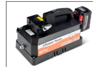
Turnkey, 10,000 PSI (690 bar) hydraulic power pump powered by an 18VDC Li-Ion battery, ships with hydraulic oil.
