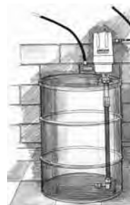
55-gallon drum mount using bung bushing
