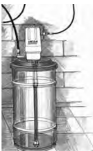
16-gallon drum mount using drum cover
