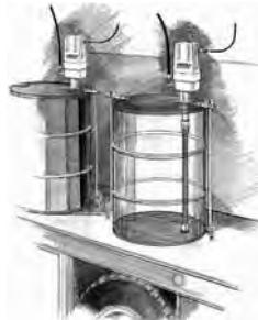
55-gallon drum mount on lube truck using drum cover
