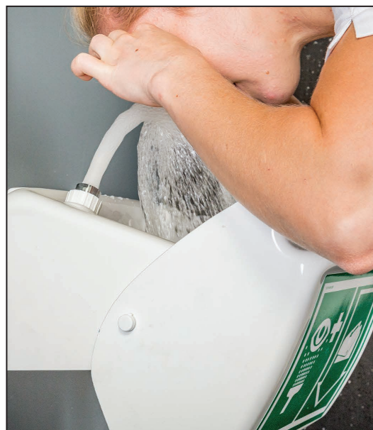
Eye/face wash stations deliver 3-gallons (11.4-liters) of tepid water per minute for up to 15 minutes to ensure a thorough decontamination.
