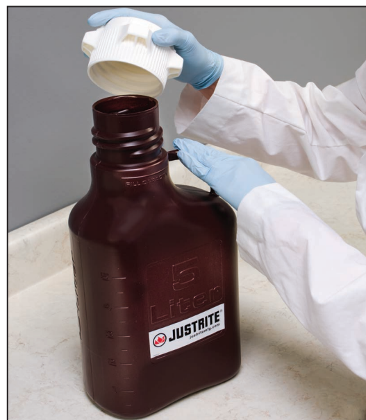
Made from a hard, opaque material, dark amber carboys offer good chemical resistance and protection from light.
