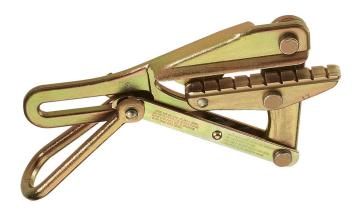
Klein Tools' 1611 Series Chicago Grips have a round inside jaw contour designed to hold weatherproof strand and solid coated wire. They also have a notched jaw to provide a firm grip on insulation. All Klein grips are manufactured from custom drop-forged steel that is machined and heat treated for excellent durability. Each grip is individually hand inspected and actuated for proper function. Grips are also rigorously tested and pulled to rated load to ensure the highest quality and reliability.
