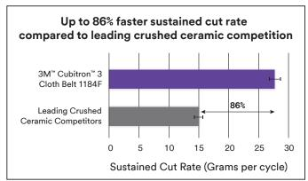
Results based on an automated, 10-minute grinding test on 304 stainless steel using 36" long belts. Error bars = 95% confidence interval. Cut rate: the total material removed in grams after 10 cycles minus total material removed in grams after 3 cycles divided by seven cycles. The unit is grams/cycles.
