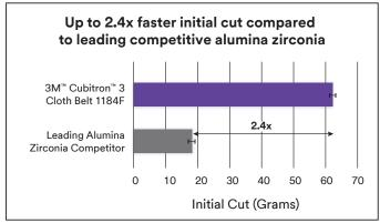
Results based on an automated, 10-minute grinding test on 304 stainless steel using 36" long belts. Error bars = 95% confidence interval. Initial cut: Total material removed in grams after 2 cycles.
