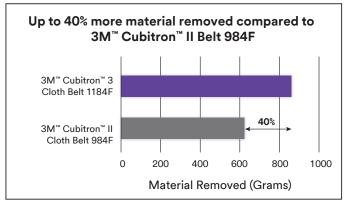
Results based on an automated, 10-minute grinding test on 304 stainless steel using 36" long belts. Total material removed: the total material removed in grams at 40 cycles.
