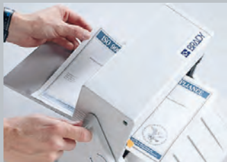
2. As it passes through the rollers, the adhesive and laminate are evenly applied.
