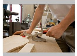
Same clamp model, same settings, Auto-Adjusts to different heights and maintains the same clamping force !!
