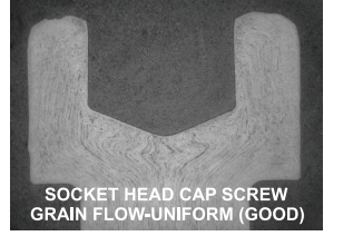
SOCKET HEAD CAP SCREW GRAIN FLOW-UNIFORM (GOOD)
