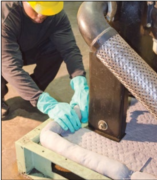
Sorbent socks mold easily around the ledge of machinery, absorbing leaking oils and overspray.
