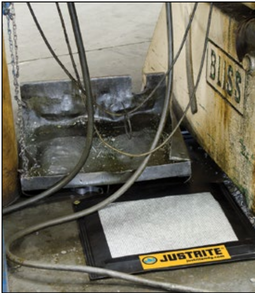
Position drip pad in tight spaces between machinery to capture oily leaks.
